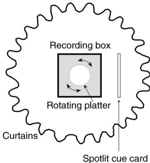
**Fig. 1** The experimental apparatus. The black curtains formed an enclosure 2 m in diameter and 2 m high, in the centre of which a square box (60×60 cm) rested on 30-cm-high supports. The circular centrepiece of the floor of the box was attached to a rotating motor and could be turned at 0.13 rpm in either direction
