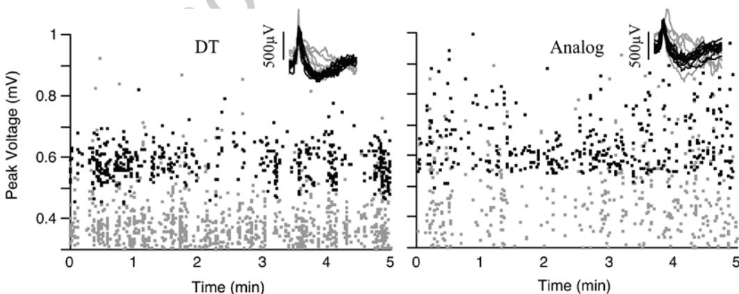
Fig. 6. DT offers improved discrimination even at the input stage. The digital signal was converted to analog and recorded by a commercial analog system for 5 min then the electrode was recorded by the conventional system. Plotting peak action potential voltage against time reveals that the discriminated unit (*black*) is less variable. The unit was also more distinct from other APs (*gray*) in the DT recording (i.e. the peak was more separate from other events).
